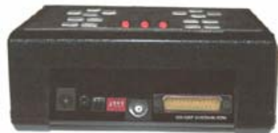
Back of Periscope Controller (KSPRC-100) Local Control. Plugs into Little Joe for Wi-Fi and Internet control
