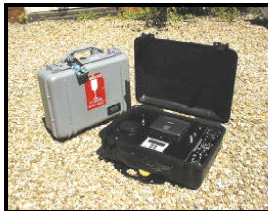
Ground Receive Case (open) with Surveillance Case
